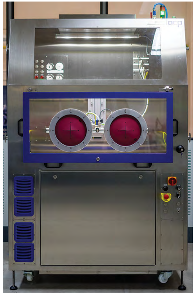
The compact, cleanroom-suitable JetStation-HP is designed for cleaning tasks involving small quantities of parts that have to meet the highest cleanliness standards. With the manual cleaning booth, parts are loaded and unloaded via a front flap with hand access.
