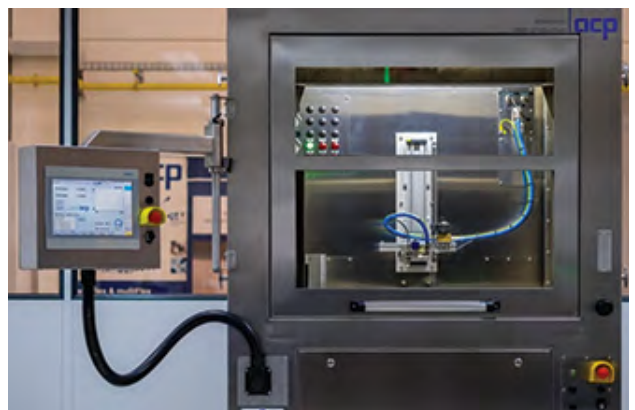
With this automated, stand-alone system made entirely from stainless steel, the part to be cleaned is placed in a receiver mounted on an x/y-axis, rotary table, or combination of both, located in the process chamber.
